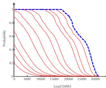
Figure 1: Load-Duration Curve and how different generation resources are dispatched to cover demand
