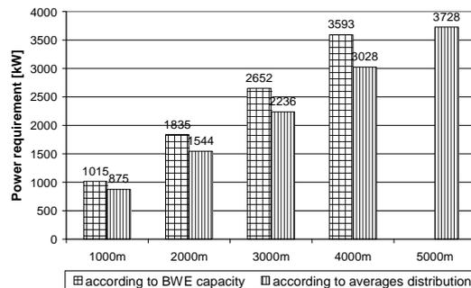
**Fig. 3:** The differences of required drive power between the standard driving force calculation (full bucket-wheel-excavator capacity) versus 97.5% quantile of averaged maximums (computed upon the recorded distribution of actual volume capacity of the BWE) (Gładysiewicz & Kawalec 2006)
