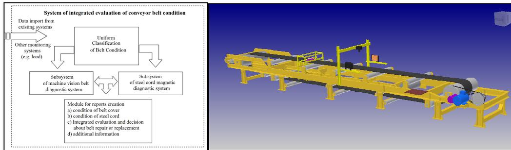
**Fig. 2:** Left: Integrated belt condition diagnostic system utilising information from magnetic and machine vision subsystems. Right: Special testing belt conveyor (Blazej & Jurdziak 2011)
