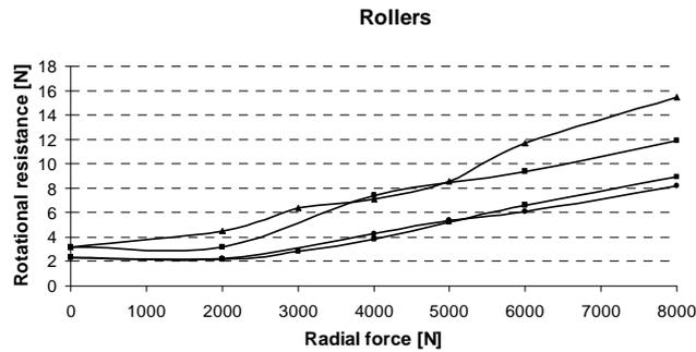
**Fig. 1:** Rotational resistance of rollers as a function of their radial loading (Bukowski et al. 2010)
