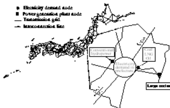
Fig. 1: Schematics of the multi-regional optimal generation planning model
