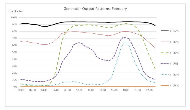
The stations in cluster 1 (which make up 22% of our sample) are running base-load, close to full output throughout the day. Those in cluster 2 also run continuously, but reduce output as load falls overnight. Cluster 3, however, turn off overnight and incur start-up costs (fuel and mechanical wear and tear). Cluster 4 groups stations that turn on for the morning peak in demand, turn down in the middle of the day and then increase output for the evening peak,
