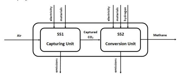
Figure 1-simplified life-cycle flowchart of the DAC-U system
