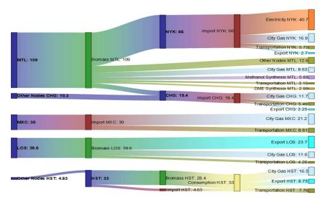
Figure 3. Modeled hydrogen production, distribution, and utilization for 2100 (MTOE)
