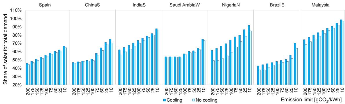
Fig. 3. The energy share of solar PV in the least-cost portfolio for the modeled regions under different carbon emission limits. The energy share is calculated as the electricity produced by solar PV (curtailment excluded) over the total electricity demand of the system.
