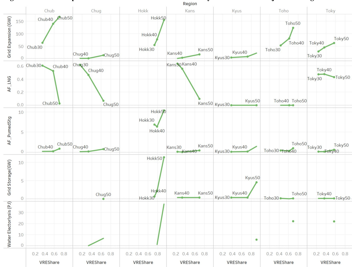
Figure 3: Relationship between VRE Share and Each Flexibility Mechanism in Major Grid Regions
