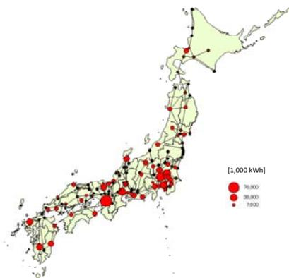
Fig.1 Power grid and demand in optimal power generation mix (OPGM) model
