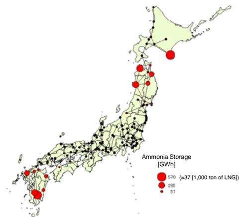
**Fig.4 Ammonia storage capacity in CO<sub>2</sub> 80% reduction scenario**
