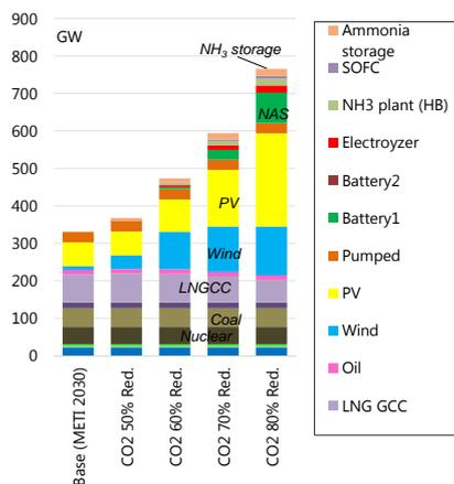
**Fig.3 Power generation capacity in CO<sub>2</sub> regulation scenario**
