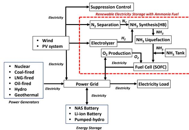
Fig.2 OPGM model combined with renewable-based ammonia storage system
