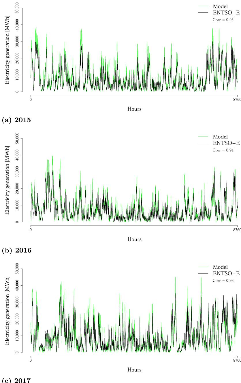
**Figure A.2: Hourly PV electricity generation in Germany provided by ENTSO-E vs. model outcome, 2015–2017**
