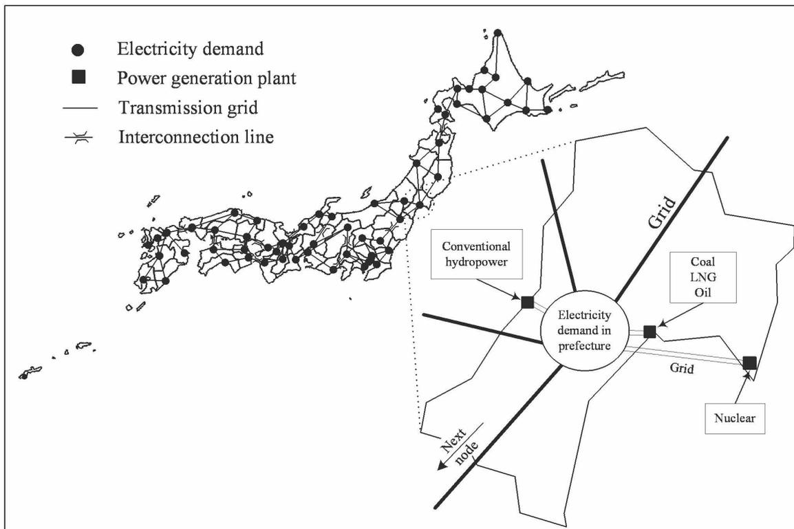
**Figure 2 Structure of Multi Node Model (MNM)**
