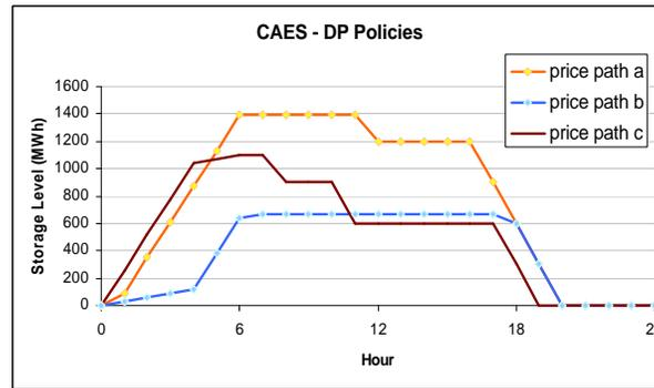
Figure 9: Optimal DP storage policies for the CAES system under the different price paths
