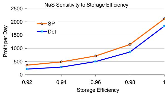
Figure 14: Sensitivity of arbitrage profits to storage efficiency of the NaS battery system
