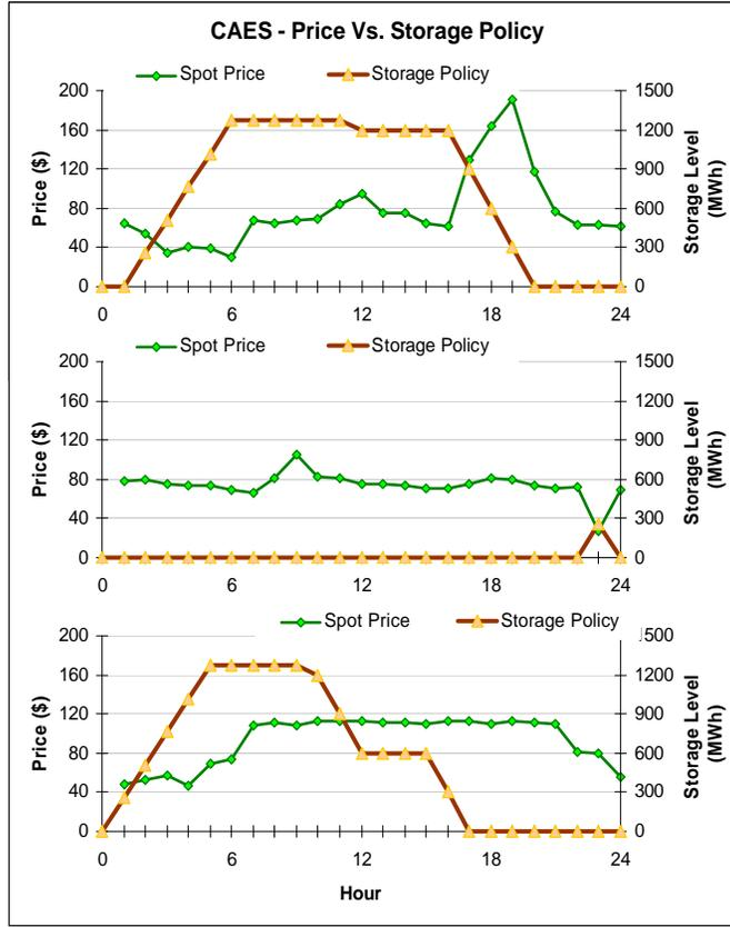
Figure 7: Optimal deterministic LP storage policies for the CAES system under different price paths. From top to bottom: path (a), path (b) and path (c)
