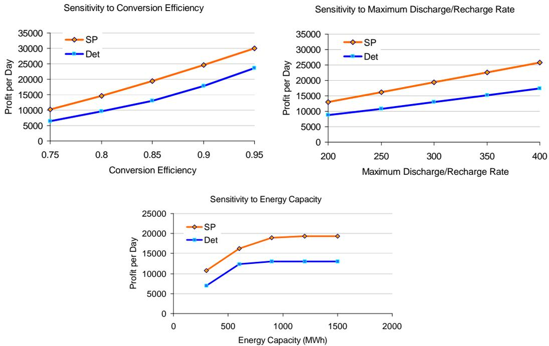
Figure 12: Sensitivity of arbitrage profits to physical parameters of the CAES system
