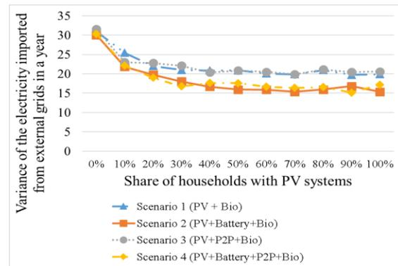
Figure 1 Variance of the electricity imported from external grids in a year, when flexible operational mode of the biogas plant is introduced in four scenarios, respectively.
