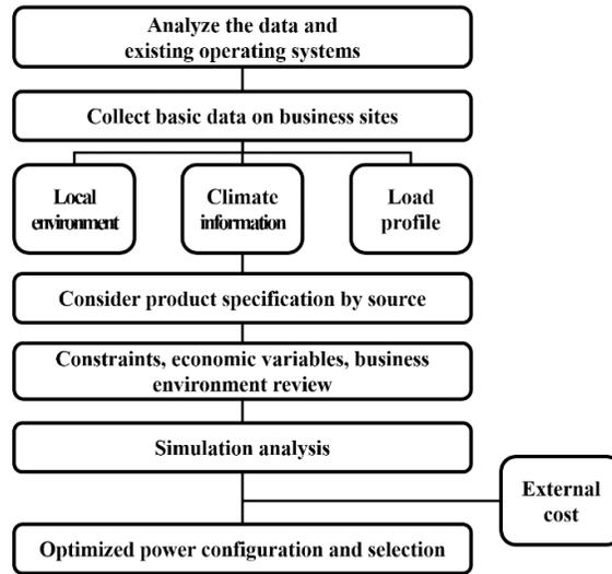
Figure 1. Energy-isolated island generation mix framework
