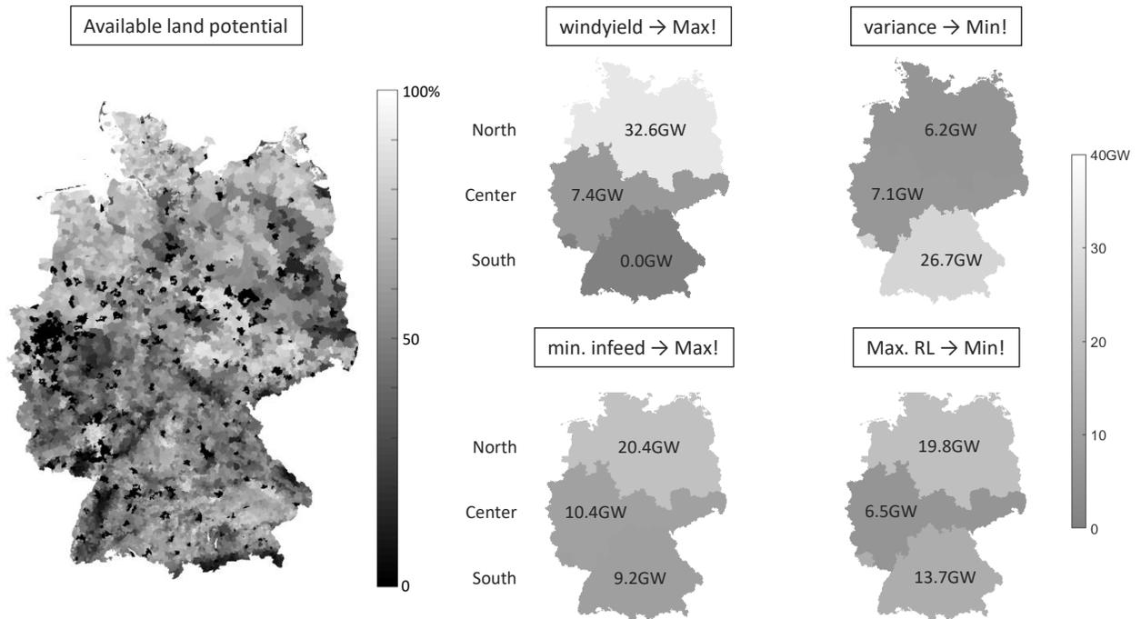
Figure 1: Available land potential in % per site and resulting wind allocation for Germany in GW per region
