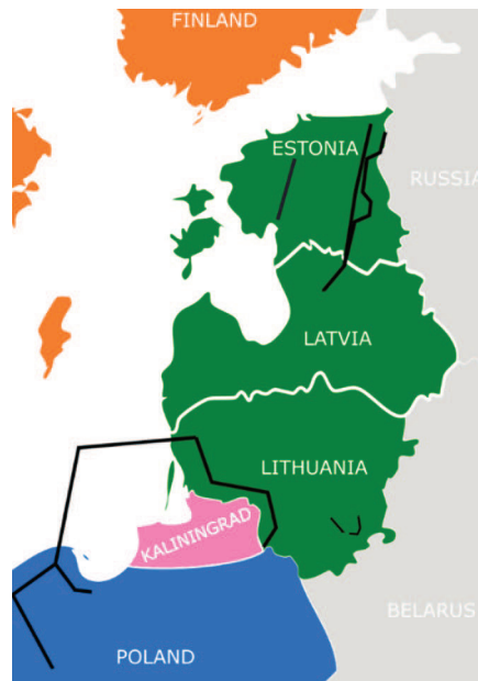
Figure 3. Baltic power system development plan (new and upgraded power lines). Source: JRC elaboration of ENTSO-E data (TYNDP, Europe's Network Development Plan, Baltic States Synchronization with Continental Europe).
