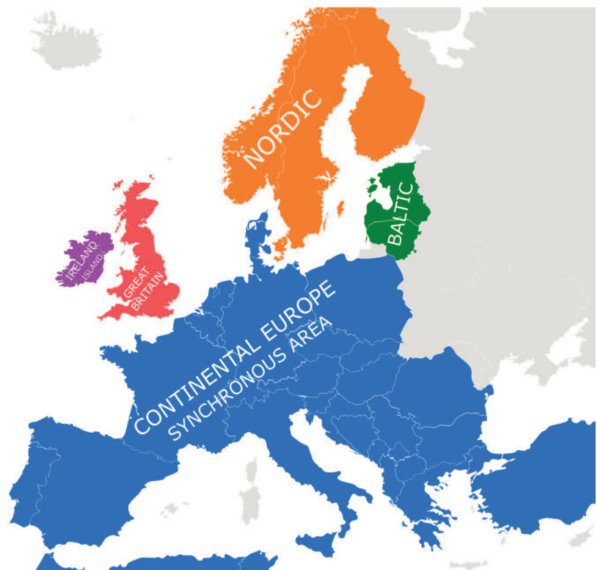
Figure 1. Synchronous power grids of Europe - the Baltic power system is part of the larger BRELL (Belarus, Russia, Estonia, Latvia and Lithuania) power grid. Source: JRC elaboration of ENTSO-E data.
