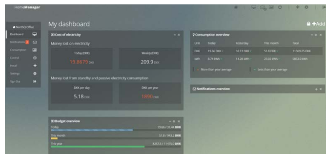
Figure 1 – Snapshot of consumption information available to SM customers online. ©NorthQ and Bager (www.northq.com). The top-left widget (“Cost of electricity”)
